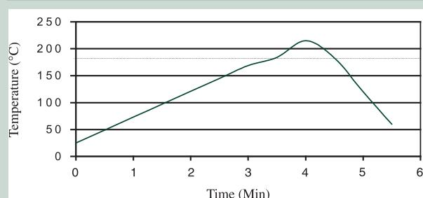
The profile shown here is designed for **Indium6.3** with Sn63/Pb37 and Sn62/Pb36/Ag2 under both air and nitrogen reflow atmosphere. It serves as a general guideline in establishing a reflow profile for these alloys.
